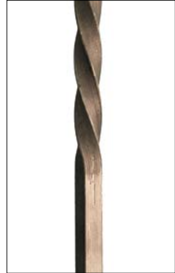
Mill scale on twist baluster
